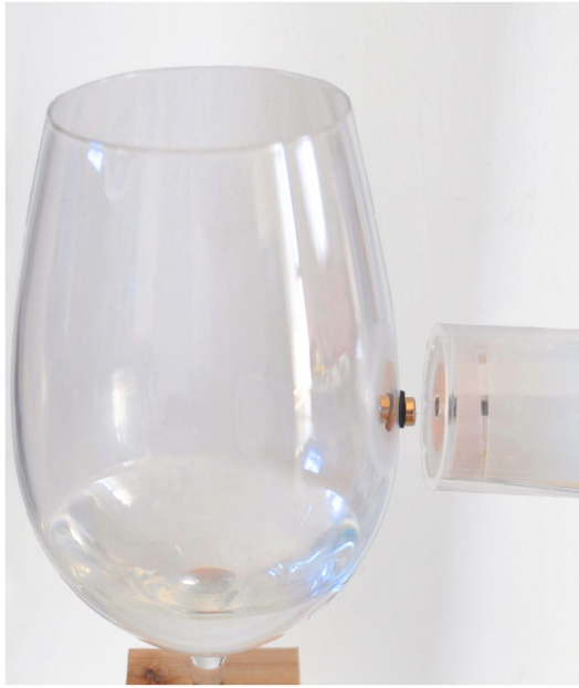
Figure 6. A wine glass fitted with two neodymium magnets, one on each side of the glass surface, padded by black foam pads. An electromagnet is placed 2 mm away from the outer magnet.
