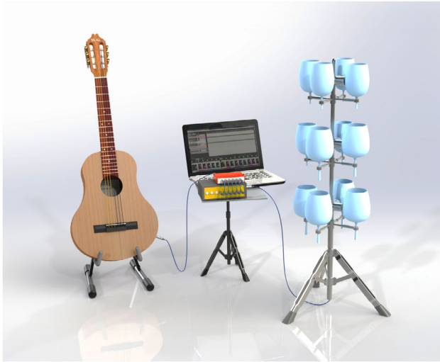
Figure 1. A proposed design of the Symbaline, played by an acoustic guitar, alongside all required system components—Audio interface, Amplification module and PC. (Guitar model: Milos Golijanin, Laptop model: Gopal Kundu).
