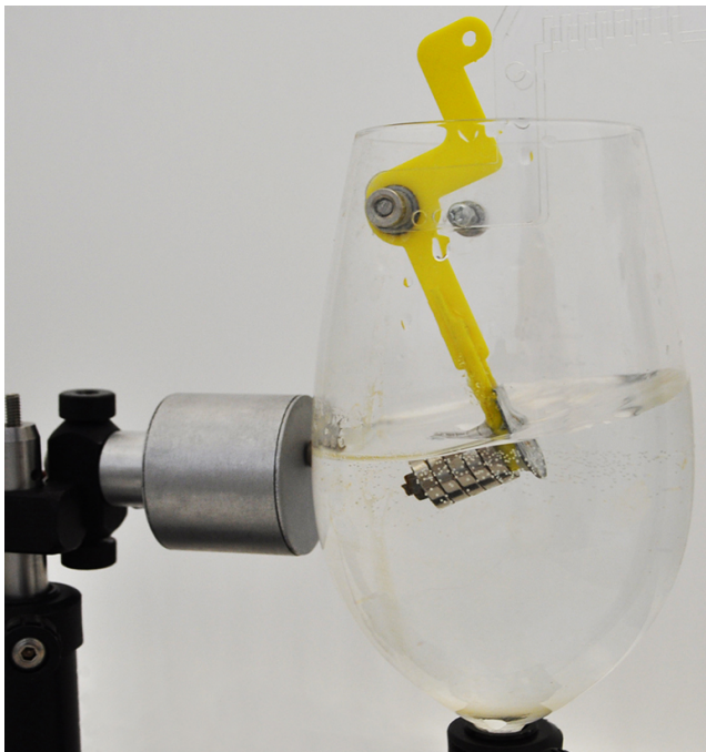
Figure 2: The modulation mechanism in mid oscillation. The pendulum is excited by the electromagnet, placed left of the glass. The water is sloshing to the right, lowering the wine glass’s pitch.
