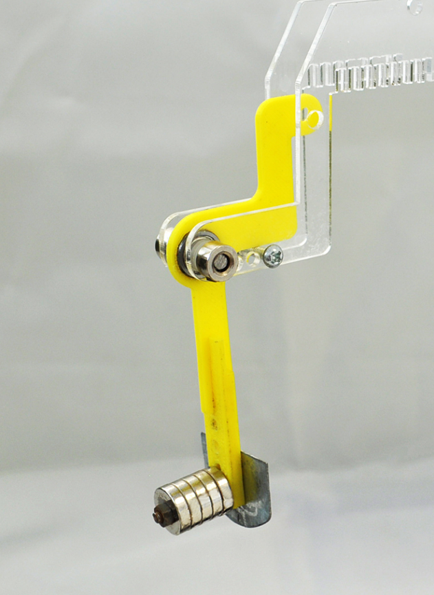
Figure 5: Closeup of the modulation mechanism, showing the pendulum, magnetic bob, blade and external supports.
