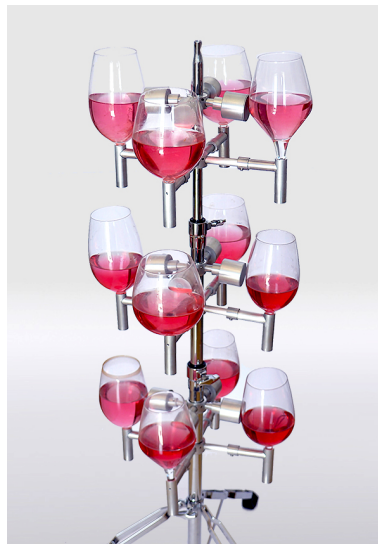
Figure 3: The Symbaline, tuned to a full octave, showing the wine glasses and electromagnets. The Symbaline is played by an amplified external musical instrument (not shown).
